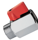
BSP male/female - PTFE seal - rode nylon handel
