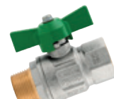
BSPT male/BSP female - PTFE seal - EPDM PEROX O-ringen - vlinderhandel
