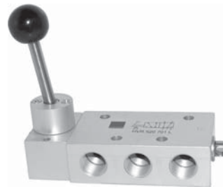
Sample Product: HVR 520 701 L Lever actuated 5/2-way spool valve, indexed, with FKM seals. Added value: The user can put a padlock in the drilling of the extended spool and thereby lock the valve.
