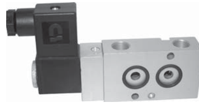
Sample Product: MNH 310 701 HT 3/2-way solenoid valve, interface according to 1/4" NAMUR-standard. Equipped with aluminum pilot-head, aluminum fixing nut and Epoxy coil. Inner seals are made from FKM.
